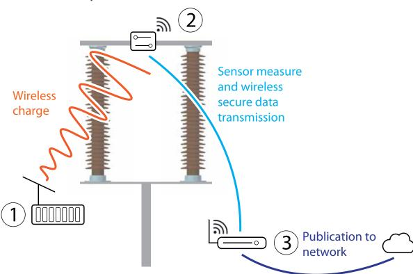
monitorWise® technology monitors disconnectors using wireless, battery-free and maintenance-free sensors in high-voltage zones. A 'Power Transmitter' (1) supplies electromagnetic waves to a 'Tag' box (2), which takes the measurements. It transmits the data in encrypted packets to the Data Transceiver (3). The Data Transceive is responsible for sending them to a database in the Cloud via Ethernet (wired or fibre optic) or using the LTE network (4G).
